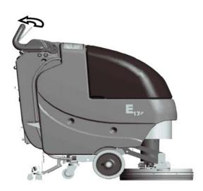
3. With the key turned on, pull the bail handle to engage the scrub brush onto the scrub deck.
