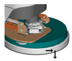
With brush removed & deck raised, Remove skirt for cleaning by pulling forward, then down over the edge of the deck.
