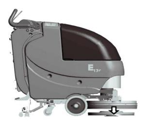
3. When done correctly the brush should release from the scrub deck and fall to the floor.
